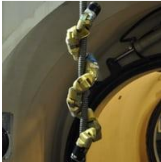
Figure 2. Helically Wrapped Modular Robotic Snake.
